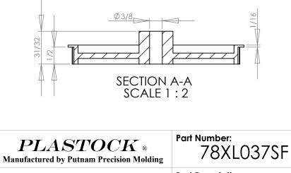
Part Description: 1/5" Pitch (XL) Timing Belt Pulleys For Belts up to 3/8" Wide
